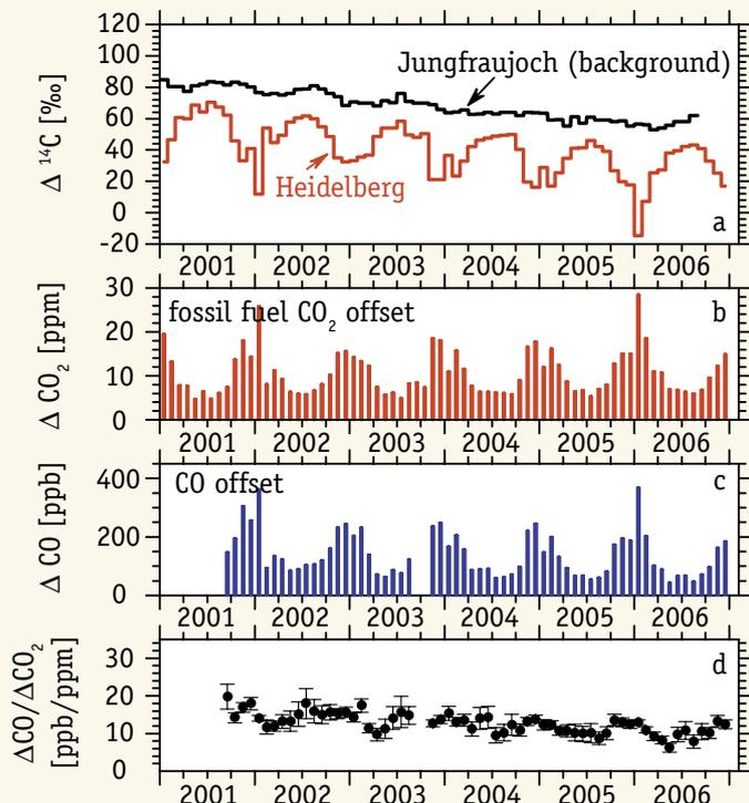
CarboEurope-IP researchers have validated the reliability of a newly developed CO-based method to calculate hourly fossil fuel CO<sub>2</sub> offsets with a number of high temporal resolution measurements of CO<sub>2</sub>, CO and <sup>14</sup>CO<sub>2</sub>, so-called "event sampling campaigns", performed in Heidelberg from autumn 2001 to spring 2003. In parallel to the event samples, two-weekly integrated <sup>14</sup>CO<sub>2</sub> measurements
