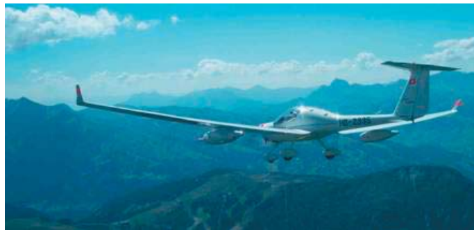
The Eco Dimona airplane, performing concentration measurements and flask sampling
